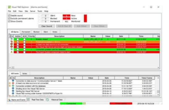
**User notification:** One of the main tasks of a SCADA system is to provide the necessary information to the right people in a timely manner. In a new SCADA system, the software administrator can assign notifications for different alarms and events to specific users or a group of users and send them email or text message notifications based on that list.
