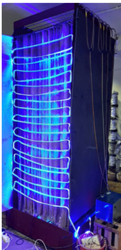
Figure 2. Pilot-scale Algal-Bacterial Attached Growth System, illuminated with blue LEDs to promote diatom-dominated biofilm growth on the textile support medium.
